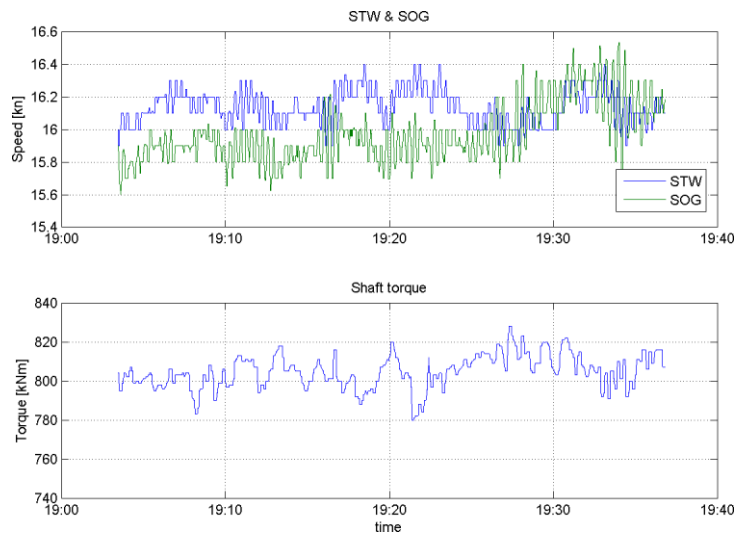
Figure 2; Speed through water and over ground and shaft torque measured on an 1800 TEU container vessel in 4 m significant wave height (Courtesy; Vroon)
