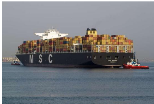
Figure 9; 14000 TEU MSC SAVONA was subjected to speed/power trials by the STA Group in both ballast draught and design draught (Courtesy: Claus Peter Offen)
